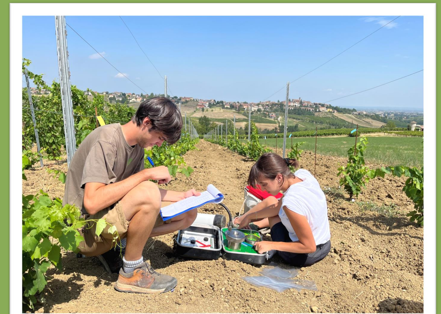
Figure 5 - A Scholander chamber was used to monitor pre-dawn (a) and midday leaf water potential (b).
